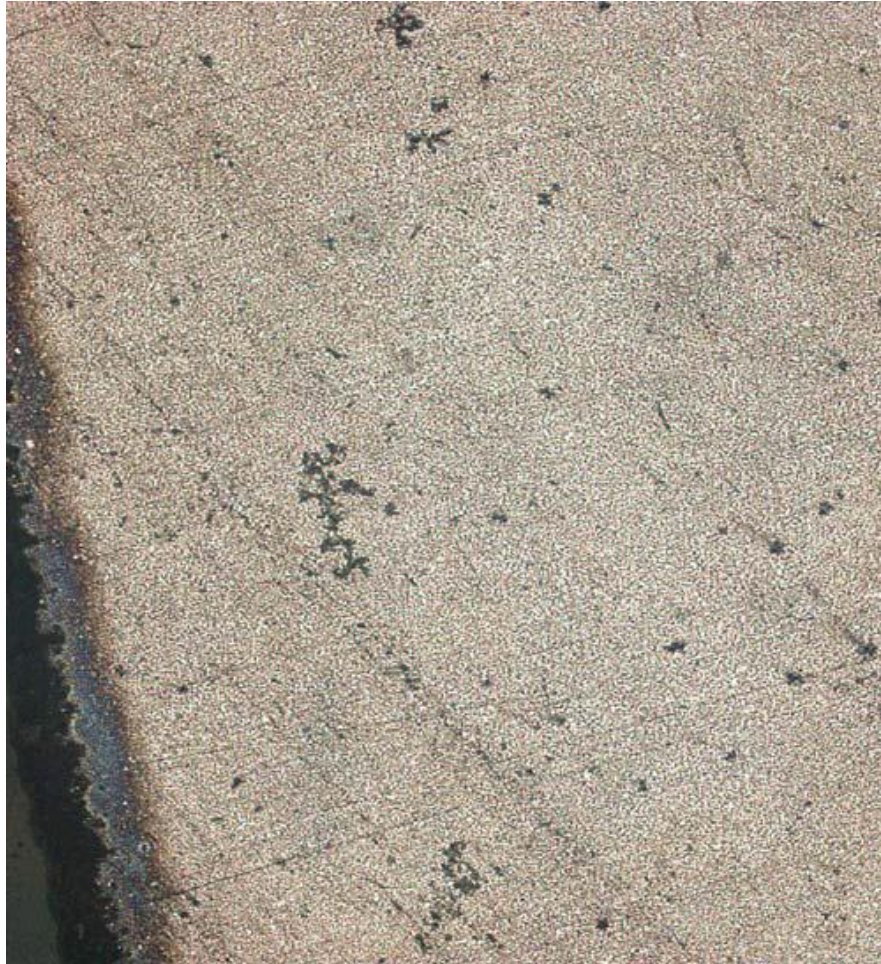
Eta-Phase in Cemented Carbide Materials 硬质合金里的ETA相
